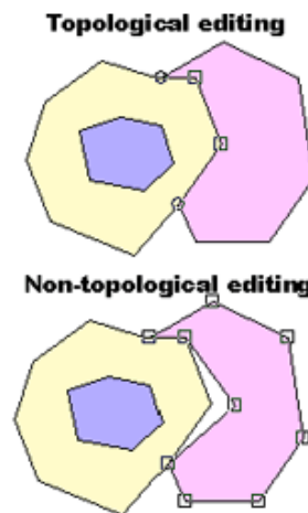
Figure 1: Topological editing (top) vs. Non-topological editing (bottom) (Theobald 2001)
