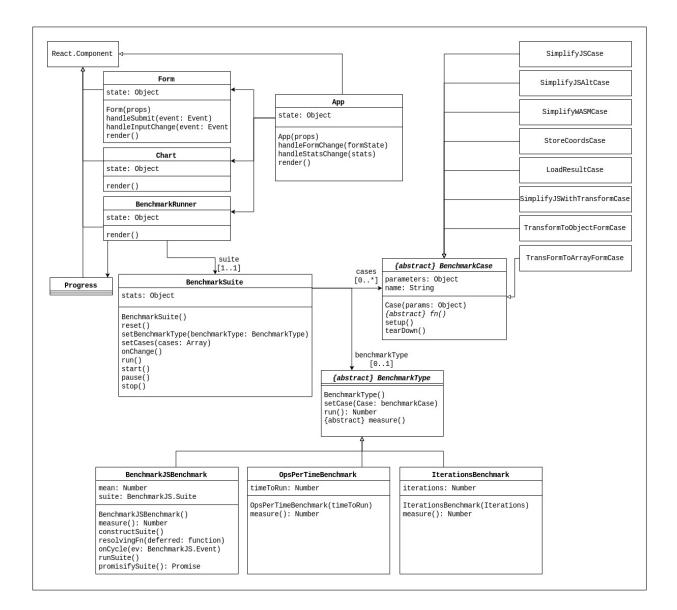
Figure 3: UML diagram of the benchmarking application
