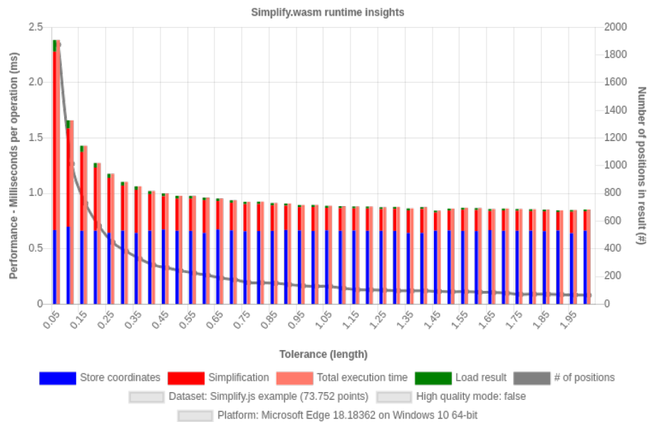
Figure 14: Simplify.wasm runtime analysis benchmark result of Windows device with Edge browser on dataset "Simplify.js example" without high quality mode.
